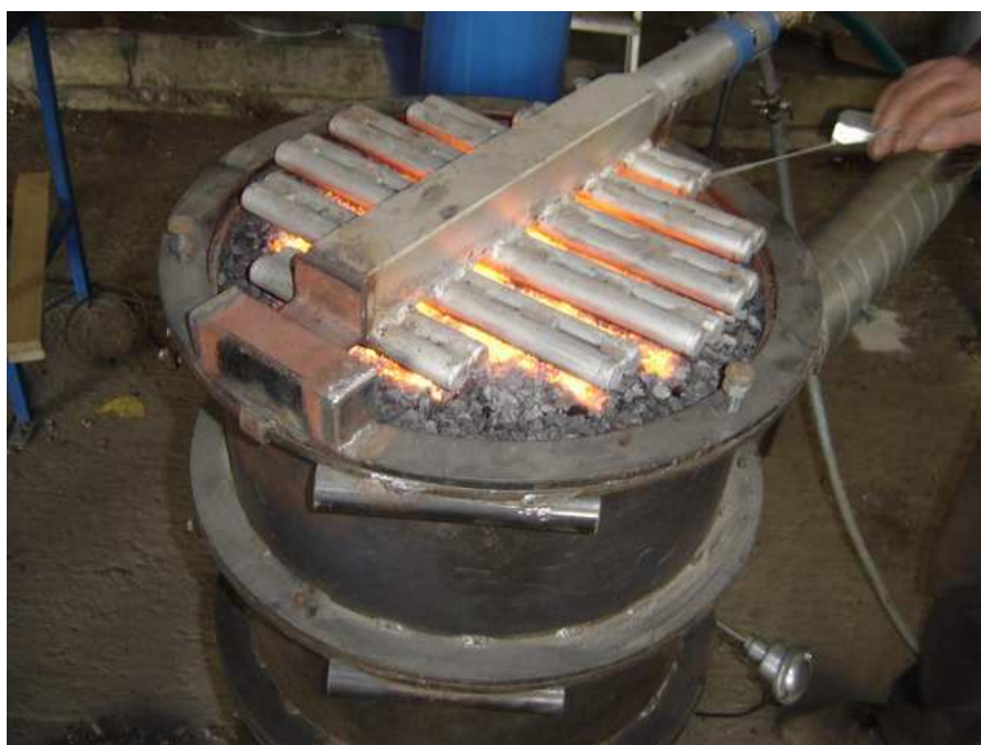
Fig. 2 Burning of the raw material charge with gas burner
