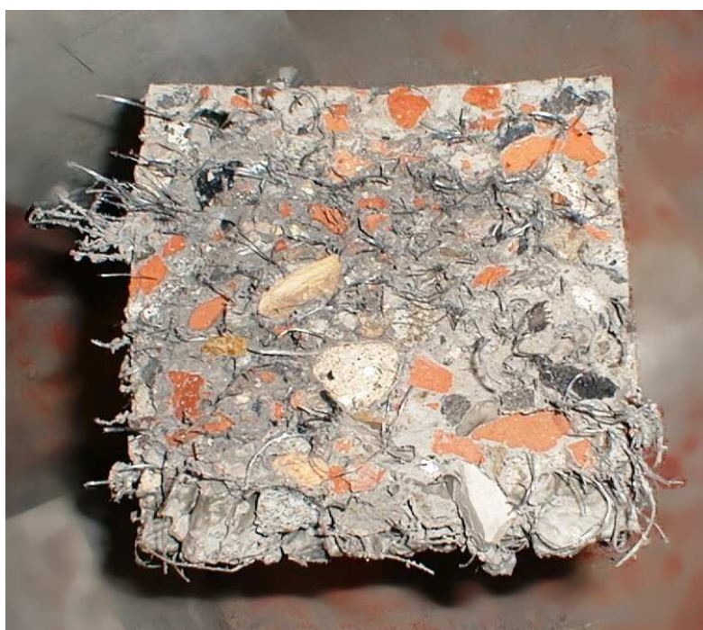
Fig. 1 Specimen with recycled aggregate and synthetic fibres after testing in the laboratory
