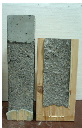
Fig. 4 Timber-OPC sample failure
