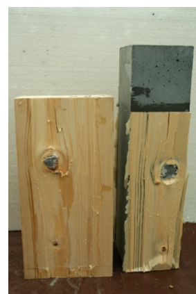
Fig. 5 Timber-UHPC sample failure
