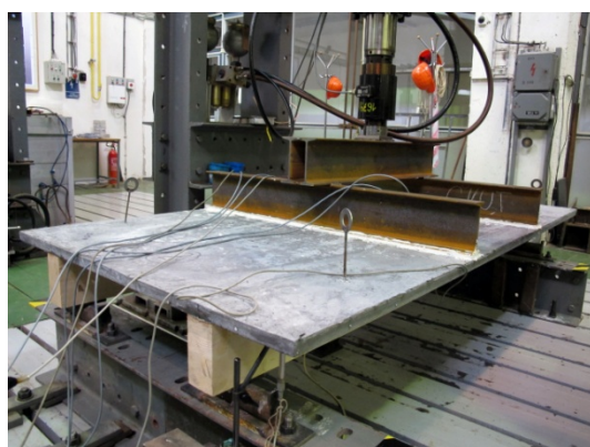
Fig. 6 Tested segment of timber-UHPC floor structure
